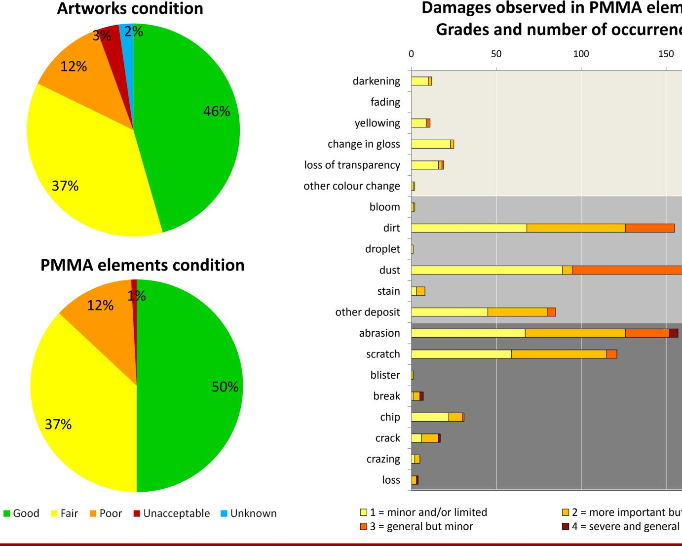
Damages observed in PMMA elements. Grades and number of occurrences.
