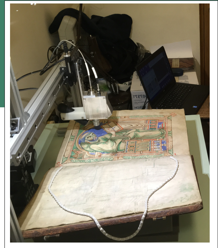
Using Raman spectroscopy to examine the c.12 "Eadwine Psalter" at Trinity College, Cambridge
